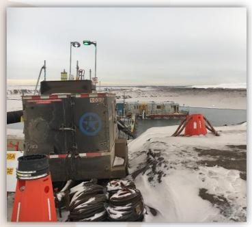
A CH15HS heater delivering hot air to a tailings barge from 500 feet away
