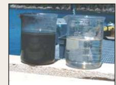
Aquaculture benthic deposit water before and after Geotube® treatment.
