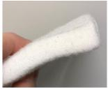
RockStop™ is a Polypropylene / Polyester protection textile with a consistent thickness throughout the width of each roll. Designed to protect the pipe during and after backfill operations, it does so by cushioning the impact and abrasion of rocks which can cause damage to the pipe. This eliminates the need to import select fill, as the on-site native soil can be used to backfill the pipeline.
